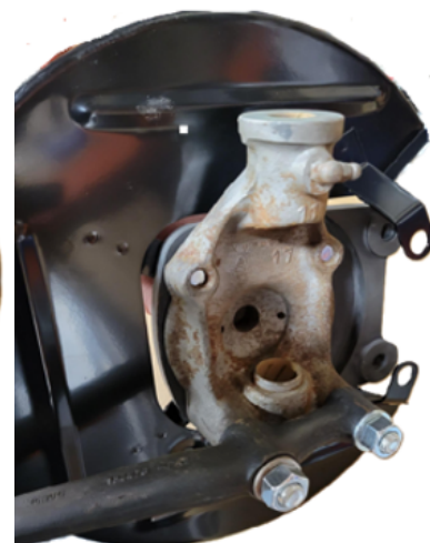
Rear view of RH dust shield loosely installed
