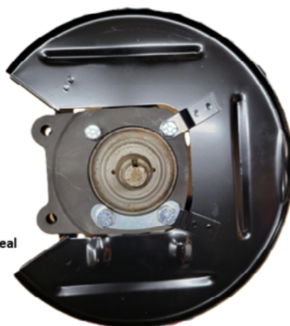
RH dust shield and fixing bolts loosely fitted
