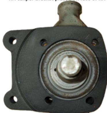
RH caliper bracket placed on face of RH stub axle.
